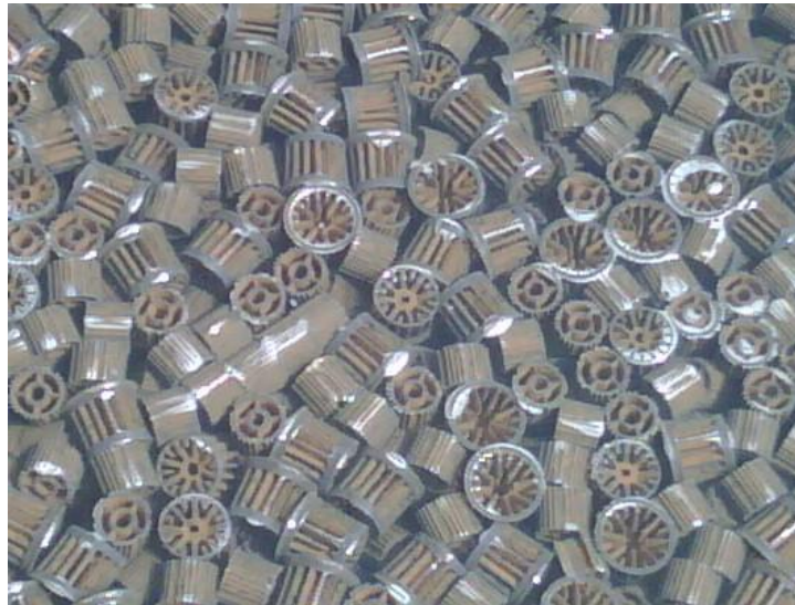
Figure: 2.07 FAB media with Biomass
